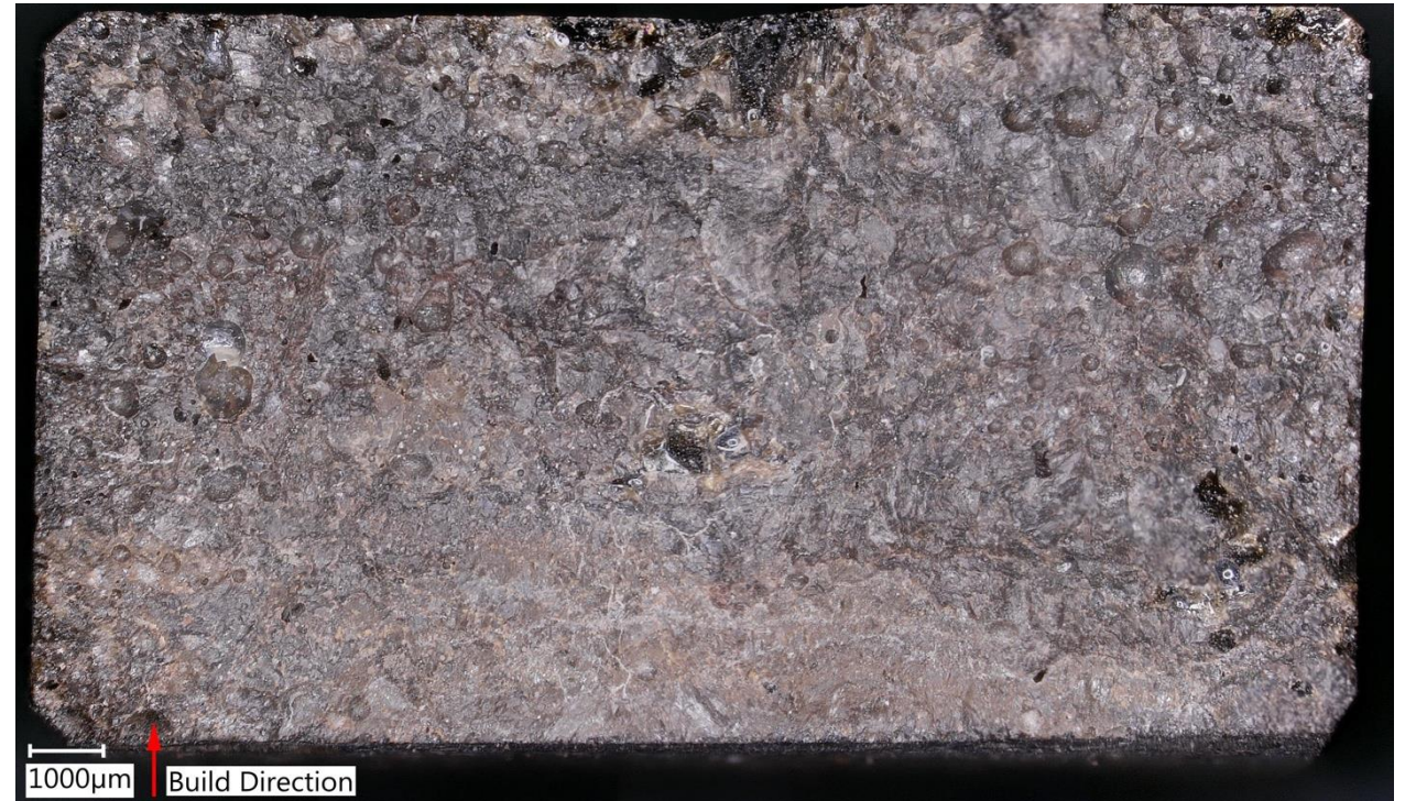
Fracture surface of specimen with flexural strength of 4 MPa
