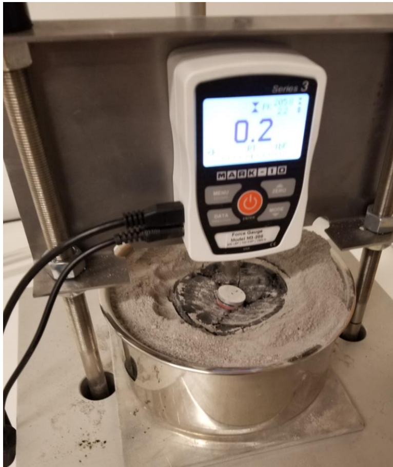
Landing pad load bearing test – 8.7 MPa flexural stress at failure
