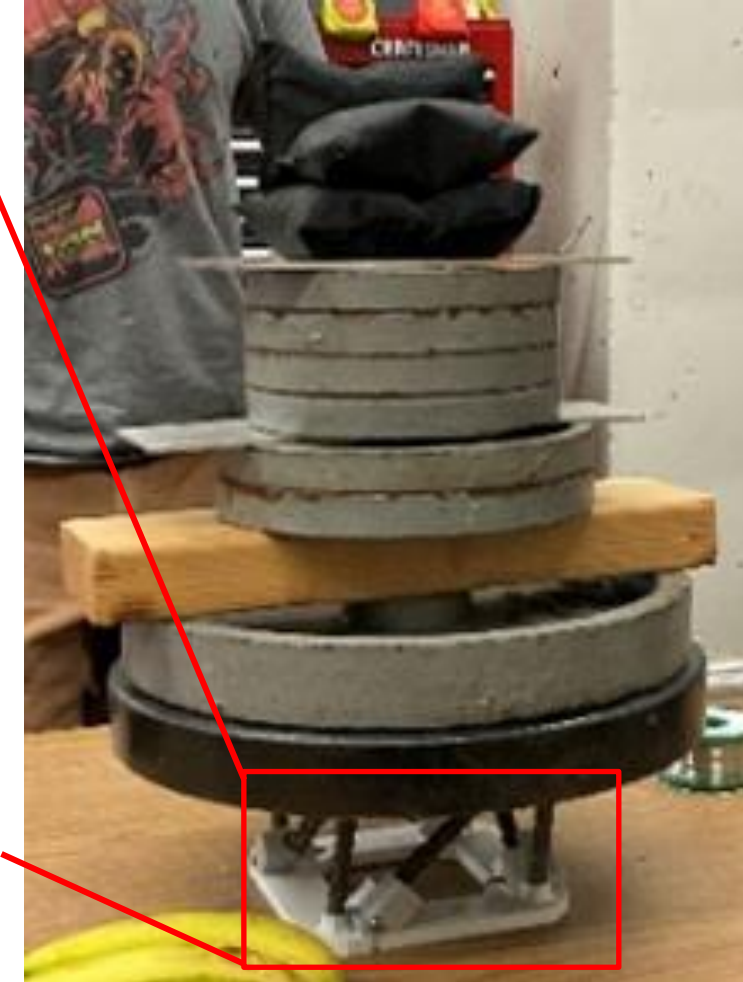
Truss assembly loaded with 34 kg before failure
